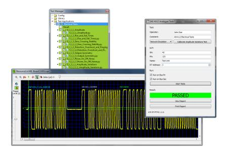
Figure 3: 1553 RT Validation Testing
