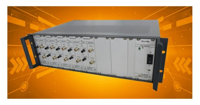
AlM's modular and scalable FOL Systems can be configured for your specific EMC or Test Bench application using an easy 'Plug and Play' approach. The units are connected by optical links using COTS 62.5/125µm multimode gradient index Fibre Optic cables with ST connectors (wavelength 1300nm).
