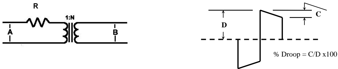
Figure 3-11 – Coupling Transformer
