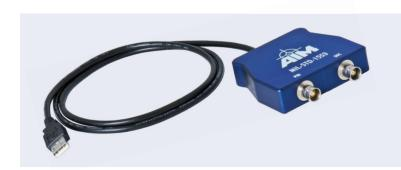
Auxiliary I/O connector gives access to 8 (avionic level) General Purpose Discrete I/O signals and 1 trigger input and 1 trigger output, plus an IRIG-B time Encoder/Decoder providing a sinusoidal input/output and 'freewheeling' mode incorporated. The SOC of the AIM SmartCable™ has access to 128MB of Global RAM and boot up flash memory.
