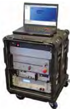
A typical Data Control and Acquisition System in a Compact rack case.
