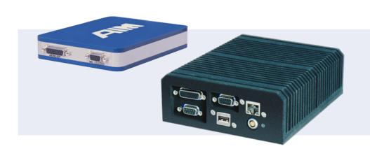
The new ANET-MxAy Mixed Protocol ANET has a maximum of 2 dual redundant MIL-STD-1553 streams and up to 12 ARINC429 channels. The MIL-STD-1553 section offers concurrent Bus Controller, Multiple RT Simulator (31) with a Mailbox and Chronological Monitor functions. All the ARINC429 channels are fully software programmable for Tx/Rx mode as well as Lo (12.5kBit/s) and Hi Speed (100kBit/s) operation.
